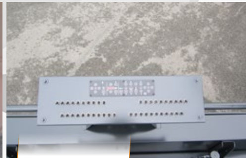
Rear platform with spraying controls
